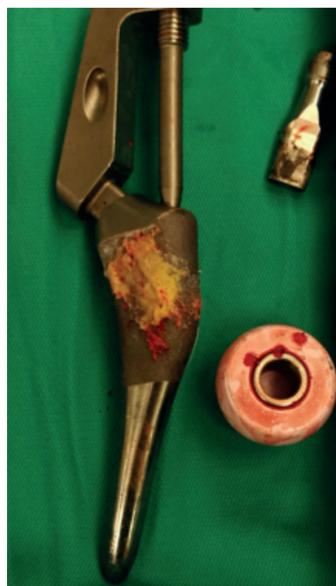
Figure 1. Metal wear due to Trunniosis.
