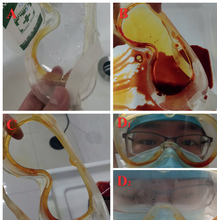
Figure 1. The way to avoid the goggles fogging. A , Wash the goggles with detergent and dry them. B , Pour the iodophor inside the dried goggles and shake the glasses to ensure that the iodophor evenly covers the surface of the goggles. C , After the iodophor on the lens dry naturally, wipe off the iodophor on the frame. D1 , The goggles treated with this method maintain a good vision after 4 hours of use. D2 , The untreated goggles fog.
